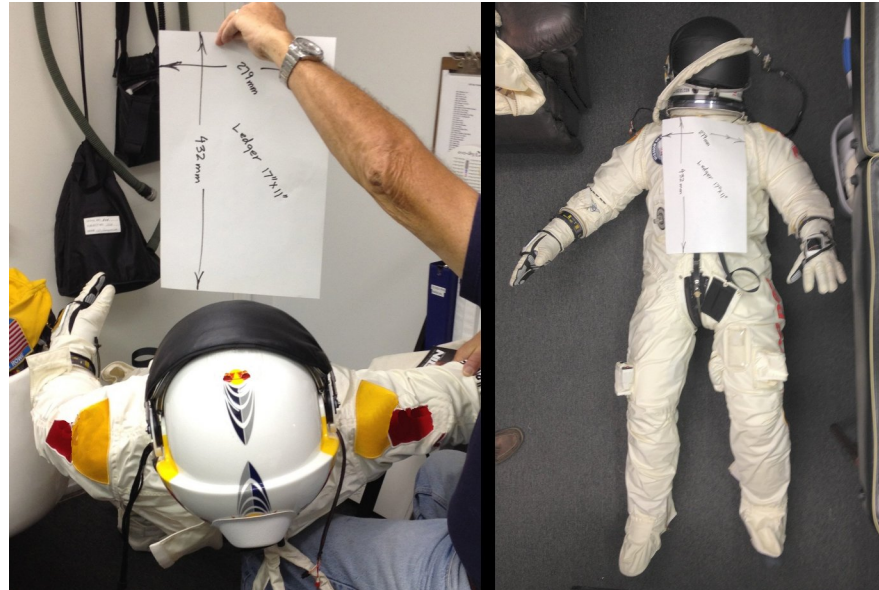
Fig 3. View of the pressure suit along the -z -axis (left) and -x -axis (right). The ledge is of size 17"x11" to determine its cross-section. (Credit: Art Thompson / Stratos team).
