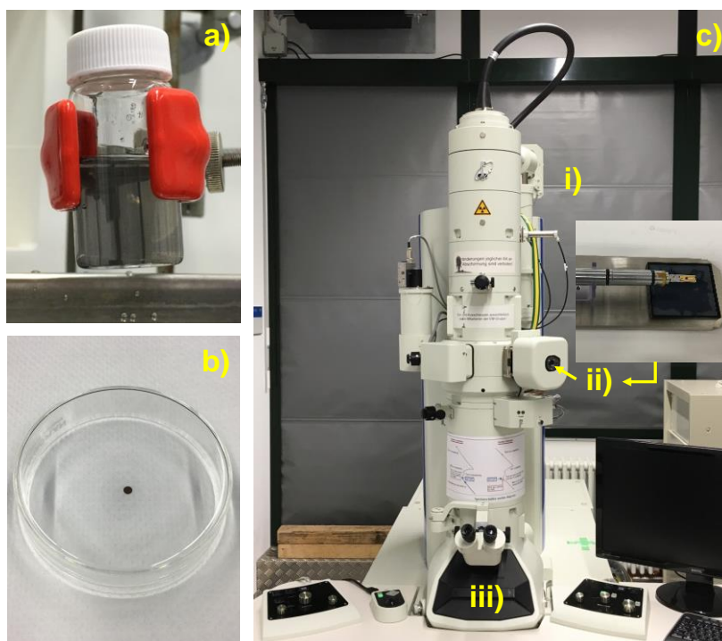
Figure 13. a) Dilute dispersion of sample; b) Copper grid with sample; c) TEM instrument; i) Electron gun; ii) Grid holder; iii) Fluorescent screen.
