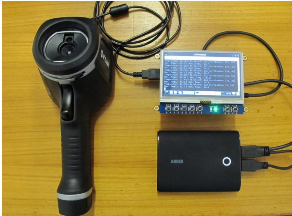
Figure 3.3: Functional test, where the proposed prototype is power supplied only by batteries.
