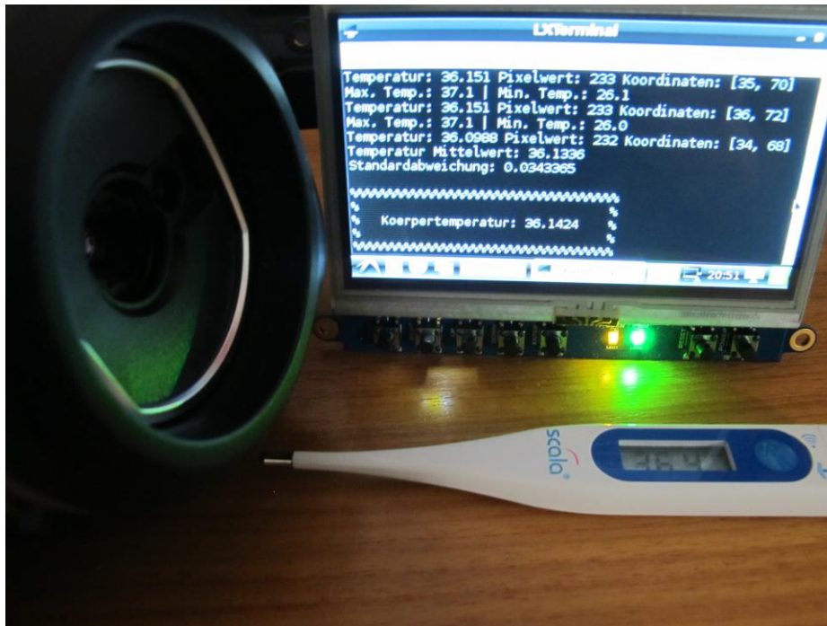
Figure 3.9: Measurement results of a medical thermometer and the thermal cam, measured automatically in a functional test.
