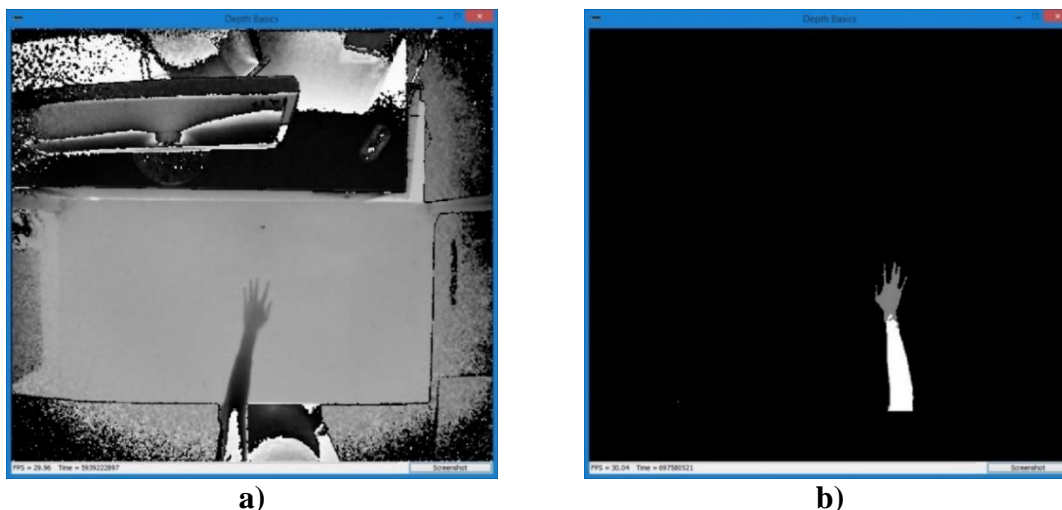
Figure 3.40: Kinect depth images. (a) The depth image from the original basic depth image example. (b) The modified version by the user interface algorithm, which cuts out all unnecessary information of the original image.
