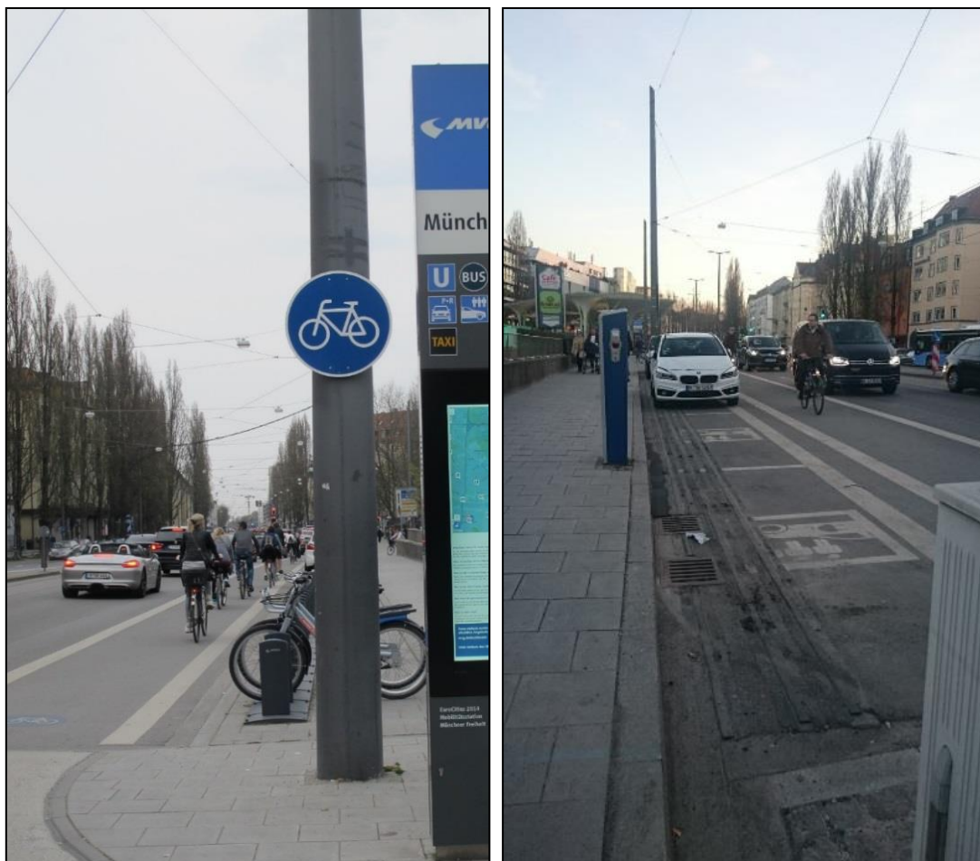
Figure 6.38: The bike lane between the reserved carsharing parking spaces and the car lanes makes parking difficult
