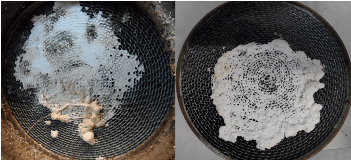
Figure 5.1: Solid by-products created at the catalyst during operating point OP2. Left: at the rear surface of the catalyst; Right: at the front surface of the ST structure.
