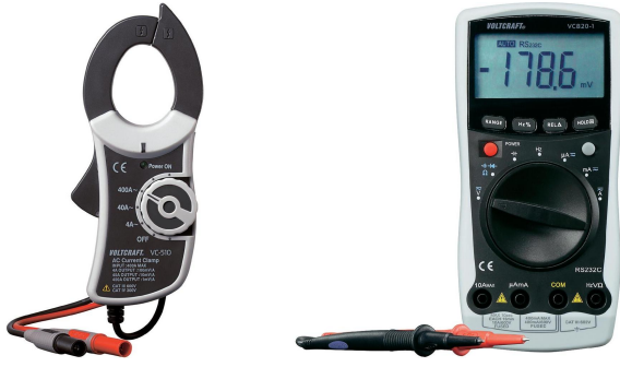
Fig. 3. AC current clamp adapter (left) and DMM (right). Source: [11]
