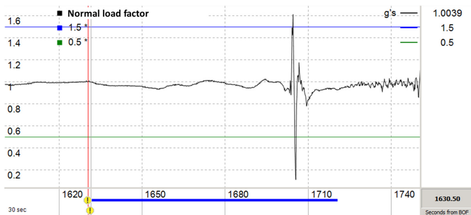
Figure 7-2 Example of load factor during a turbulence encounter (wake vortex turbulence), source: FDA
