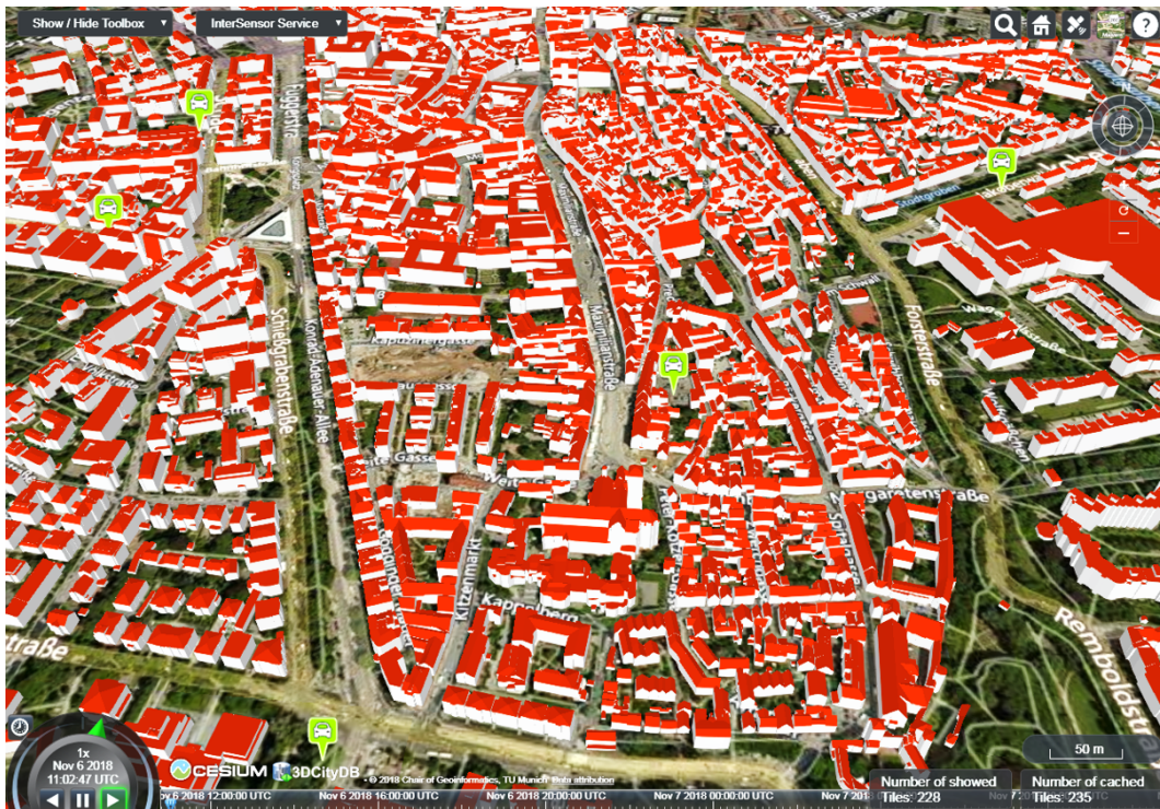
Figure 11. Joint visualization of available rental car information being retrieved by the InterSensor Service along with CityGML-based 3D building objects in the city of Augsburg in Germany. Screenshot taken from 3DCityDB-Web-Map application [91].
