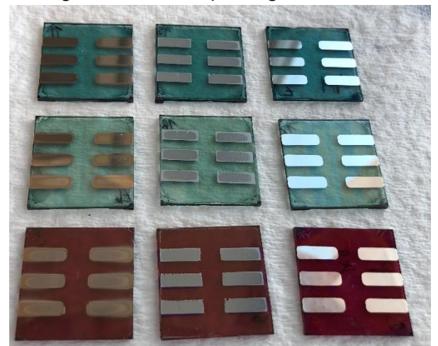
Figure 2: Solar cells with silver electrodes made from (left to right) spray coating, screen printing and evaporation.
