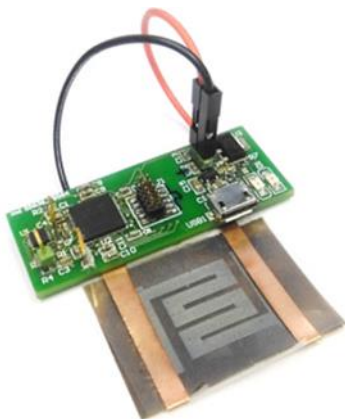
Figure 2. Resistive sensor for temperature measurements based on Laser scribing of Graphene oxide.
