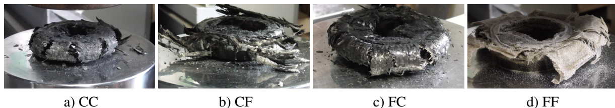
Figure 5. Crushing Modes, Photographs after Quasi-Static Compression of all Configurations
