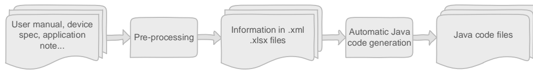
Figure 5.4: The generation flow of the device-related information
