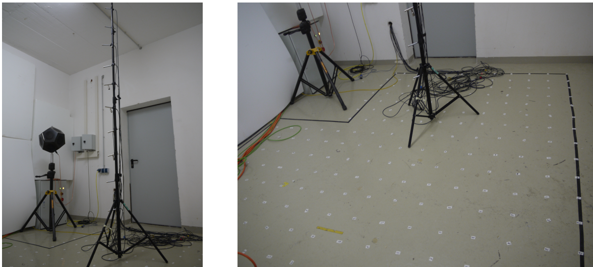
Figure 5.9: Microphone tree (left) and measurement points (right)
