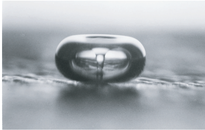
Figure 3.4: Photograph of a liquid jet produced by a collapsing cavitation bubble [86].
