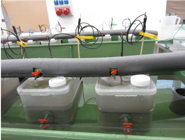
Fig. 3.1a. Photograph of two substratum-filled experimental boxes constantly supplied with natural water from the Moosach River using a drip-system and placed in a glass-fibre reinforced plastic-channel filled with overflowing water from the experimental boxes.
