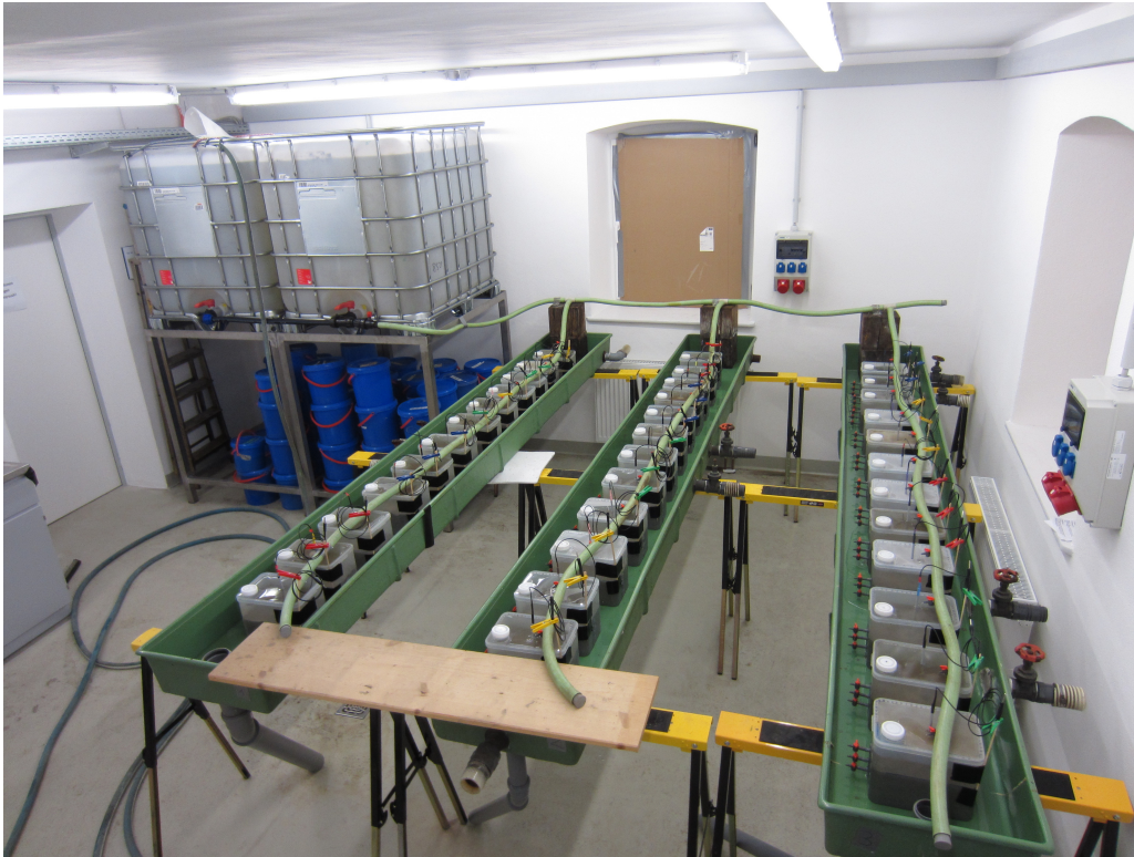
Fig. 2.2: Overall experimental setup. On the left are two 1000 l tanks filled with water from the Moosach River that is pipelined to each of the microcosms, put randomly in the artificial flow channels (green).
