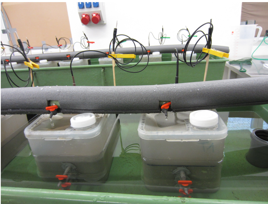
Fig. 2.3: Two microcosms constantly supplied with water from the Moosach River by a dripping system via a pipeline system (dark grey) and therein installed control valves (red).
