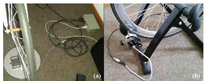
Figure 2. Recent construction of the sensors of the bicycle simulator at the Chair of Traffic Engineering and Control (Technical University of Munich), with (a) steer angle and, (b) speed value acquisition.
