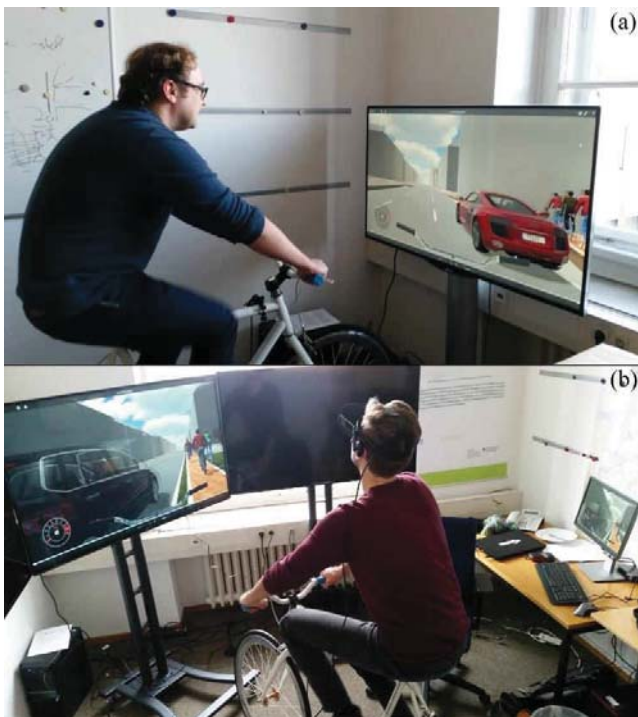
Figure 5. First bicycle simulator tests with test subjects experiencing the simulator environment with (a) one monitor, and, with (b) VR glasses.
