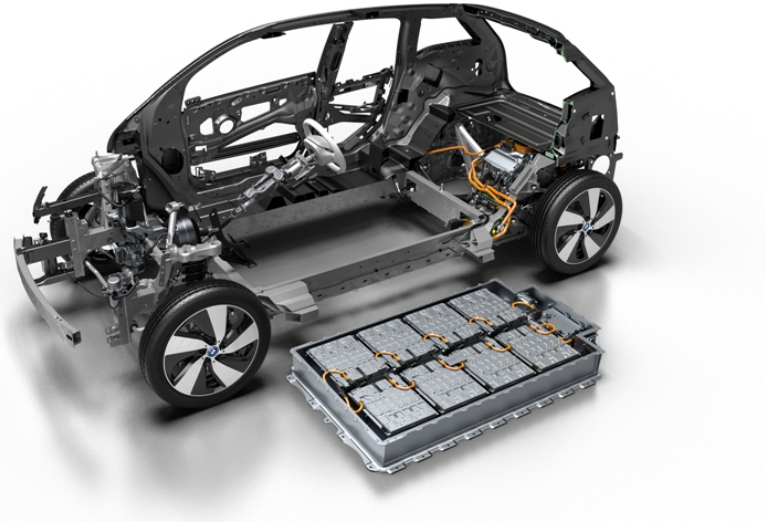
Figure 1.4: Positioning of the high voltage battery and electric motor in Battery Electric Vehicle (BEV).
