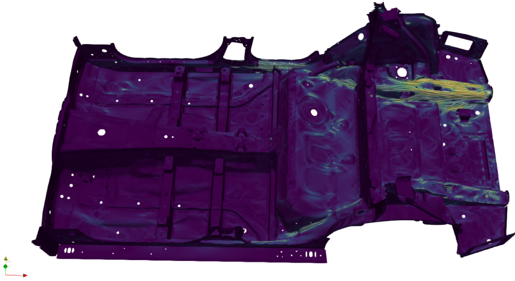
Figure 7.1: The LIC visualization: the color scale indicates the intensity of the load flow (yellow color tone represents higher magnitude of the vector field) while the texture depicts the orientation of the vector field.
