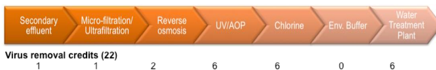
Figure 9. Virus log-removal efficiency by a potable water reuse treatment train consisting of integrated membrane systems followed by advanced oxidation processes and an environmental buffer.
