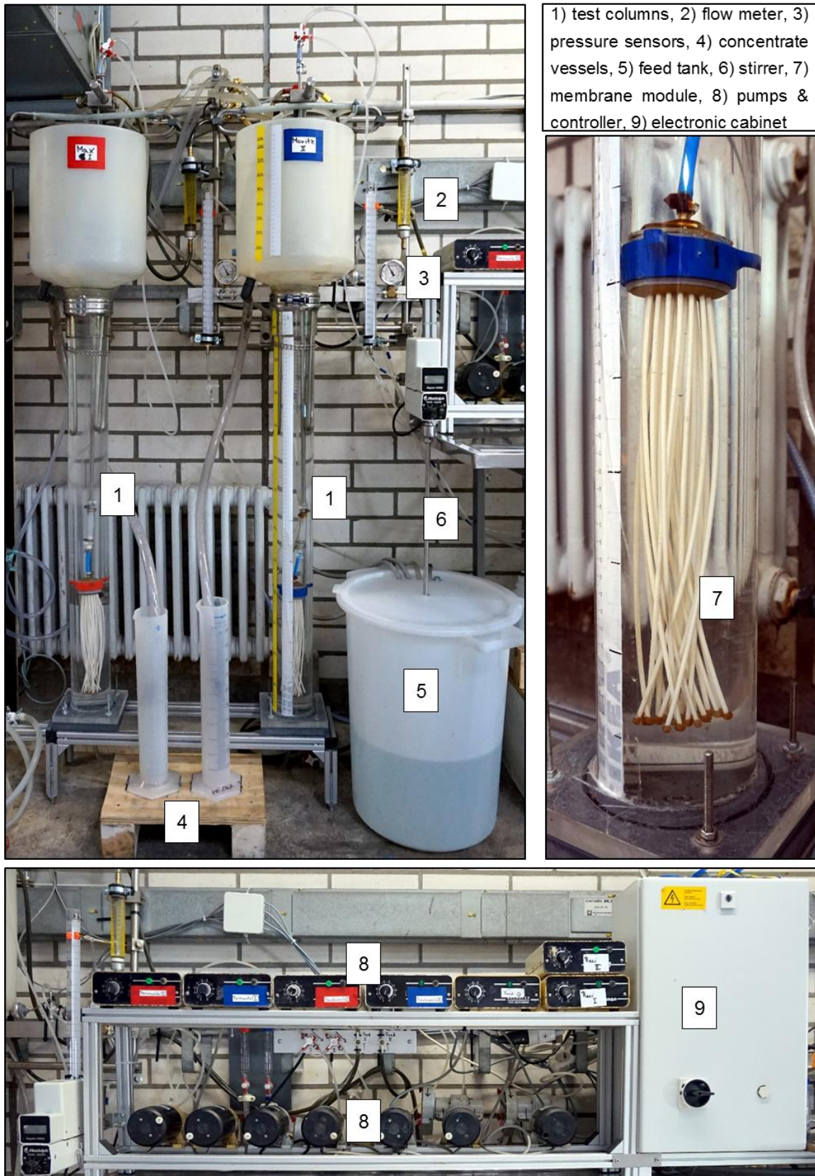
Figure SM2. Ultrafiltration (UF) hollow-fibre laboratory-scale test-skid.
