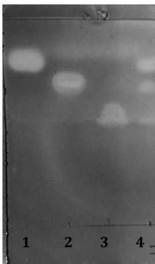
Figure 3-5: Thin layer chromatography for the qualitative detection of DAME, DA and DDA
