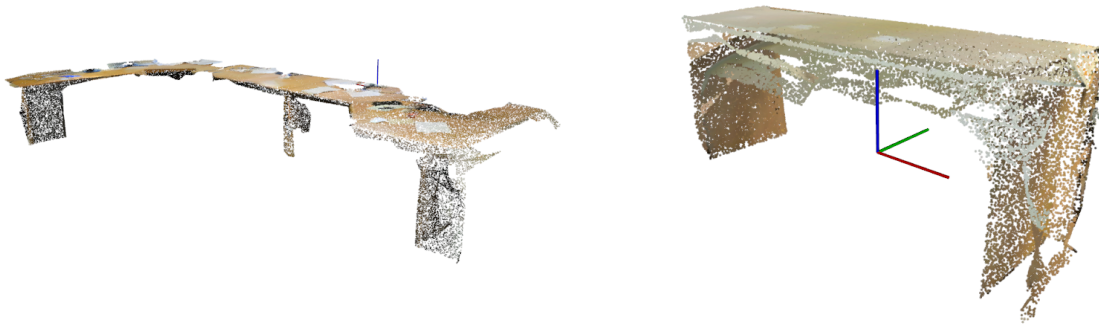
Figure 5.8: Illustration of the PC data for two instances (left and right) of object table from the Stanford dataset [11]. Significant variations in geometry between the two instances can be observed.
