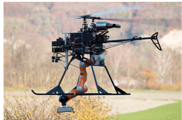
(a) Heli-manipulator system developed in DLR
