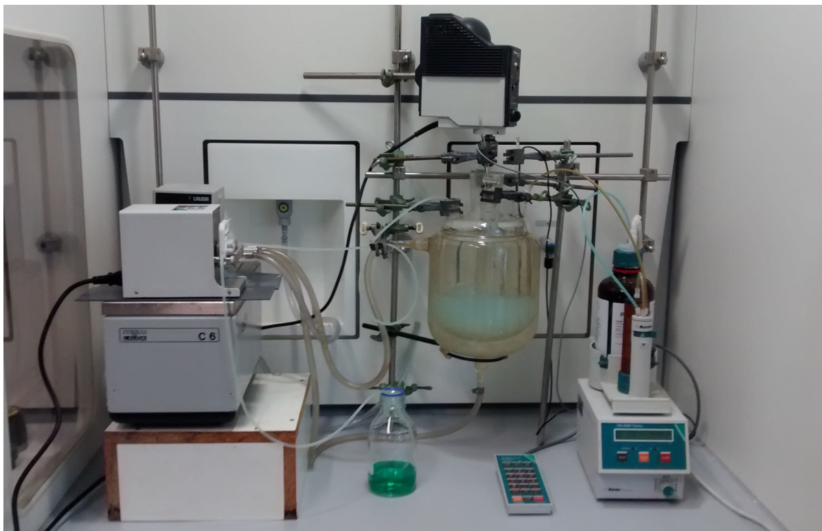
Figure 3.1: Setup for co-precipitation of Ni-Al catalysts.
