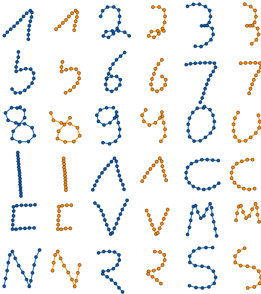
Figure 2.13: Cutting off the ends of strokes.
