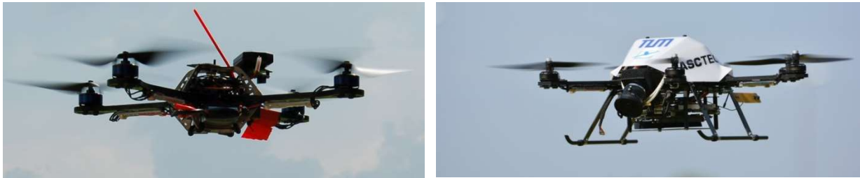
Figure 6-1: Quadcopter Hummingbird (left) and Hexacopter Firefly (right) as used at FSD
