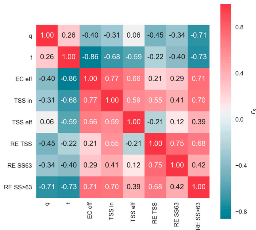
Figure 4. Correlation matrix of Spearman’s rank correlation coefficients r_s of full-scale sedimentation tank monitoring; q = mean inflow ( L s^{-1} ha^{-1} ), t = water temperature in tank ( ^{\circ}C ), EC eff. = effluent electrical conductivity ( \mu S cm^{-1} ), TSS in = influent TSS ( mg L^{-1} ), TSS eff = effluent TSS ( mg L^{-1} ), RE TSS = removal efficiency of TSS (%), RE SS63 = removal efficiency of SS63 (%), RE SS63 = removal efficiency of SS > 63 (%), n = 15 for SS63 and n = 23 for all other parameters.
