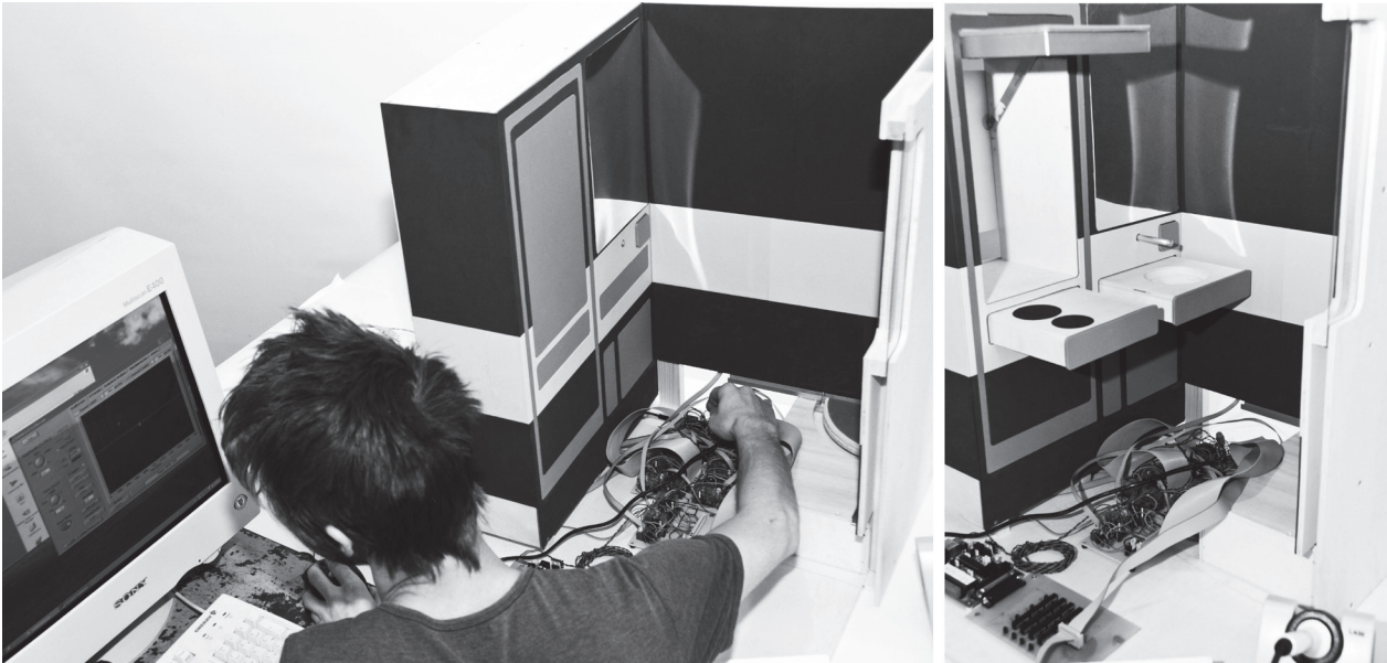
Fig. 3 Fully Functional Experimental Models of Intelligent Service Units (Room-in Room Type) The model scale is 4:1. It implements the functionality shown in Fig.1
