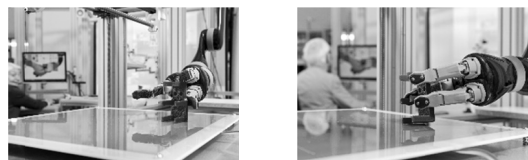
Fig. 4. Manipulation of objects with Kinova’s JACO robot.
