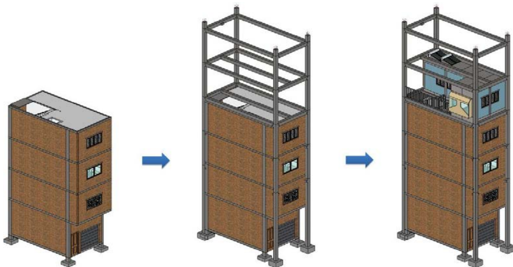
Fig. 5. Vertical extension strategy of the existing building
