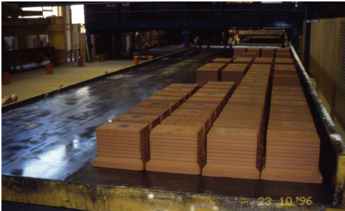
Fig. B.18: automated horizontal brickwork layering robot station
