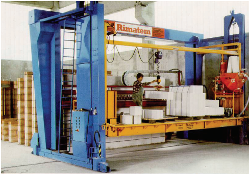
Fig. B.7: Highly flexible stationary lifting platform, Rimatem
