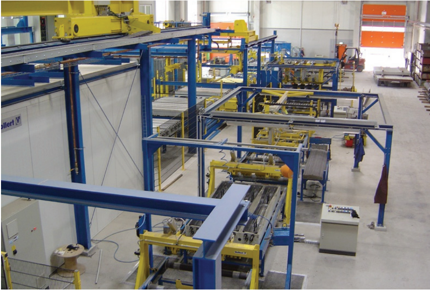
Fig. G.28: Automated track sleepers production unit (1) (Vollert GmbH + Co. KG, 2006)
