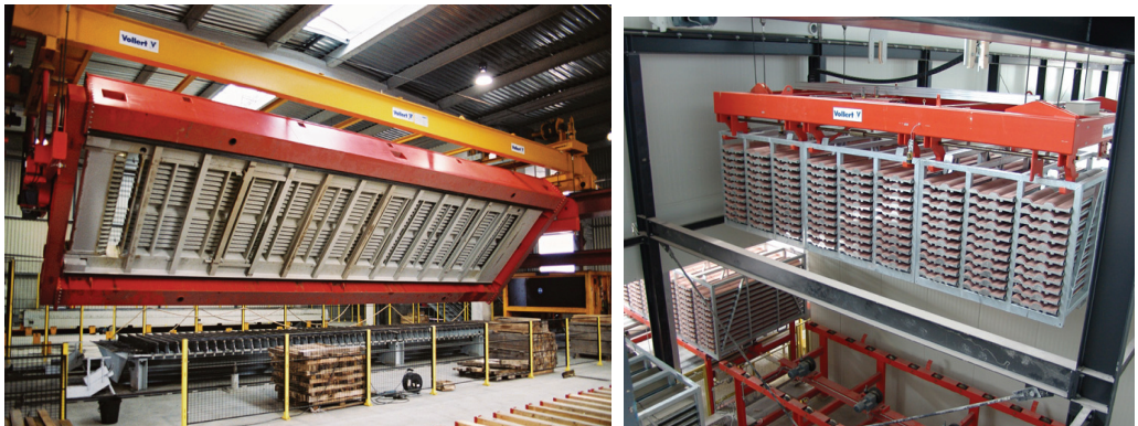
Fig. G.19: Production of concrete roofing tiles (Vollert GmbH, 2006)
