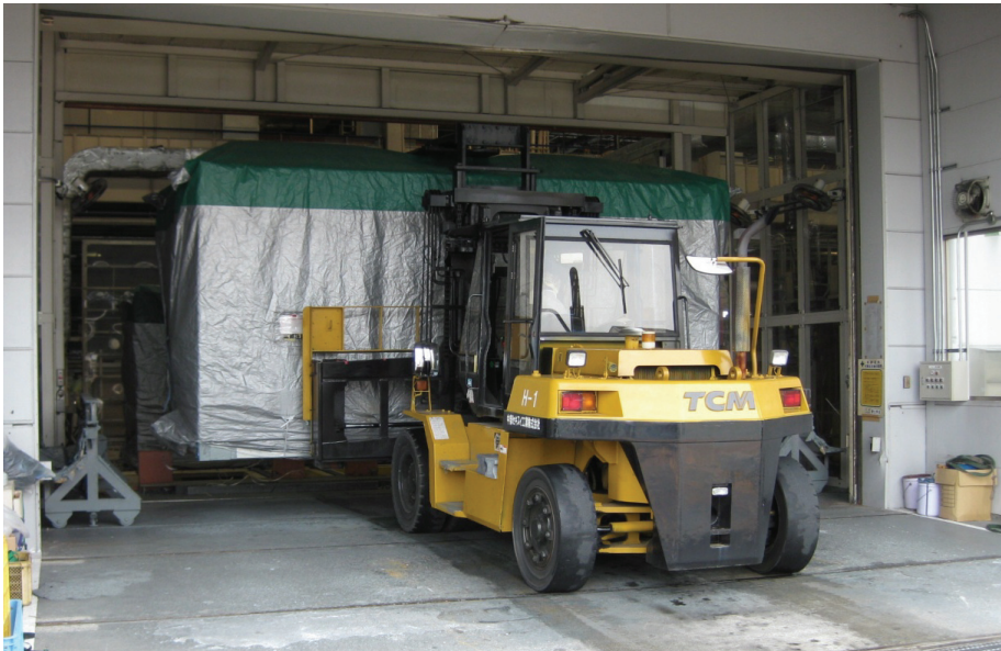
Fig. H.12: Modular building construction Sekisui Heim, completed and packaged module leaving the factory
