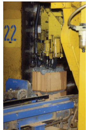
Fig. B.12: mortar dispensation
