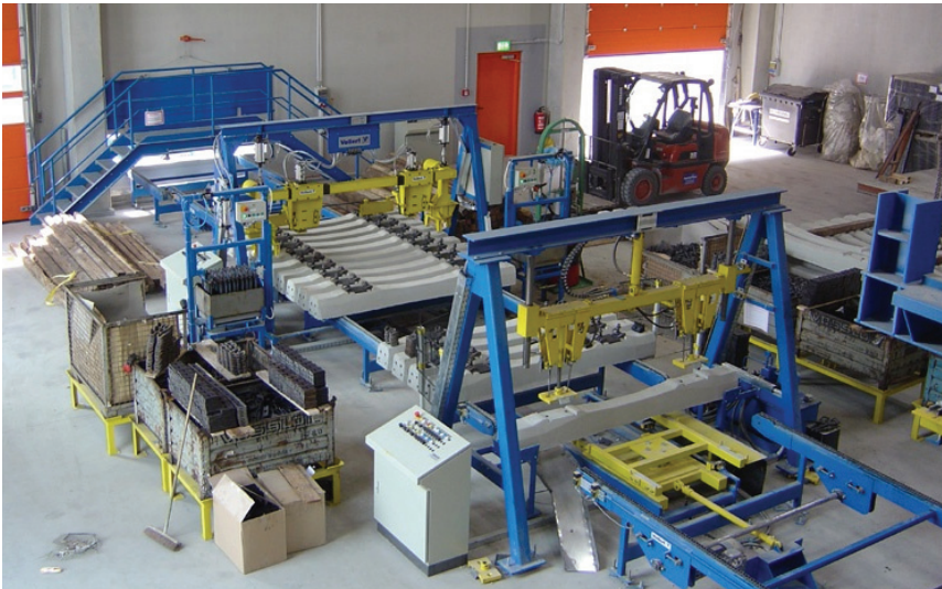
Fig. G.29: Automated track sleepers production unit (2) (Vollert GmbH + Co. KG, 2006)
