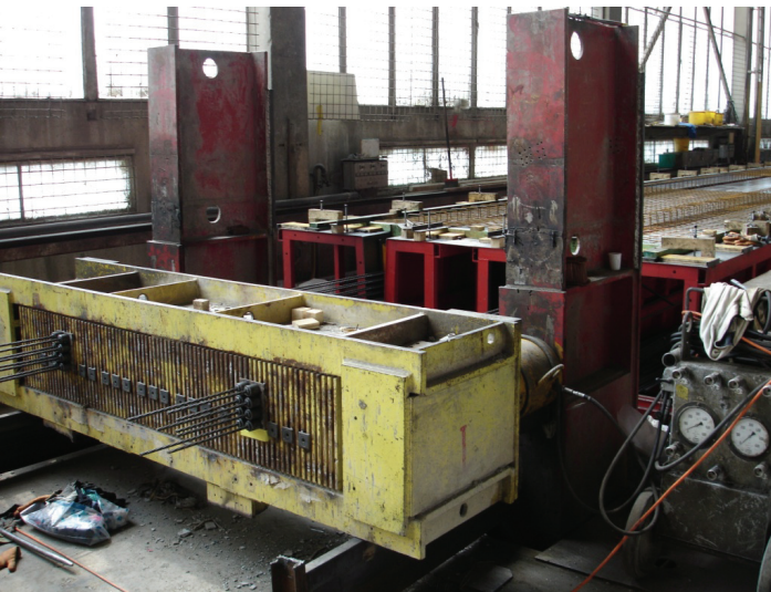
Fig. G.10: Using hydraulic presses and transoms to apply tensile force (Element AG)
