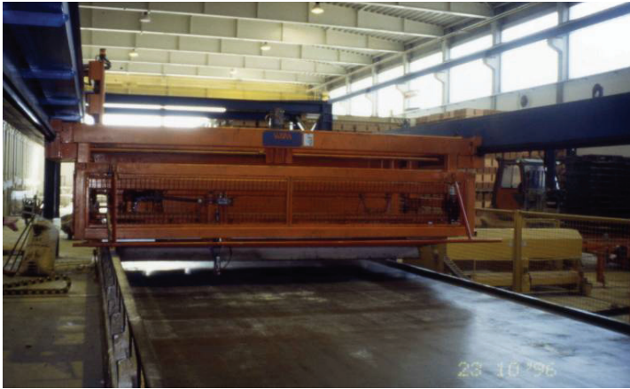
Fig. B.16: automated palletizing system with robot for distribution of bricks
