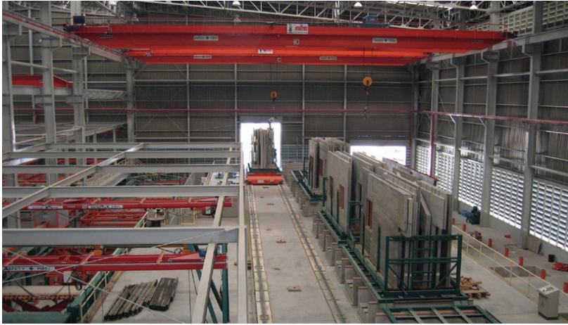
Fig. G.26: Automated crane and rail transport (Vollert GmbH + Co. KG, 2006)
