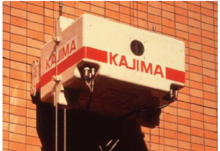
Fig. I.3: façade diagnostics robot;
