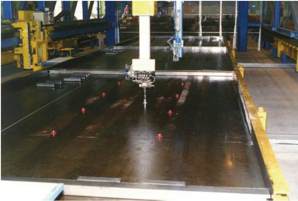
Fig. F.1: Insert Robot – Setting of a screw socket
