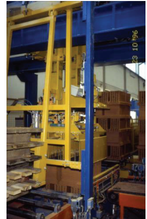
Fig. B.17: automated de-palletizing system
