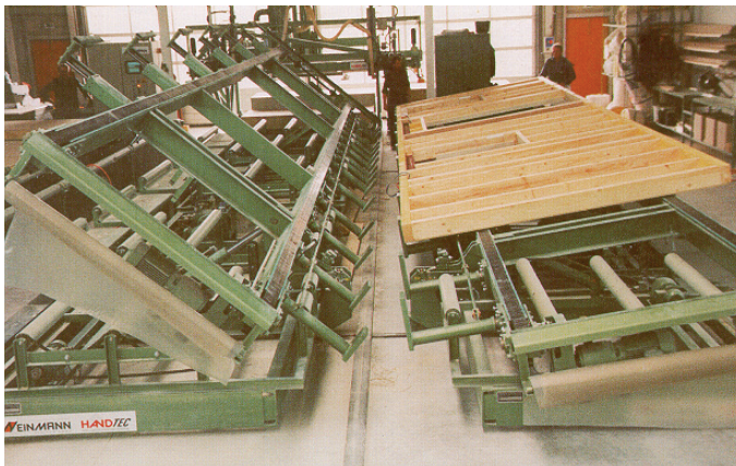
Fig. H.7: Butterfly turning table
