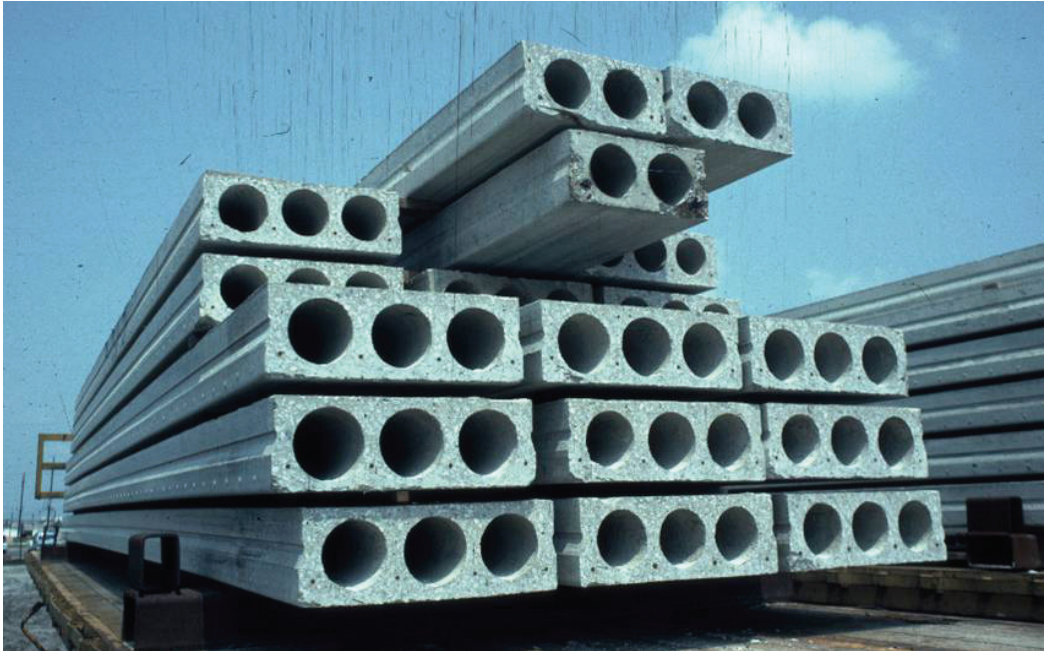
Fig. B.5: Hollow Core Prestressed Concrete Slabs
