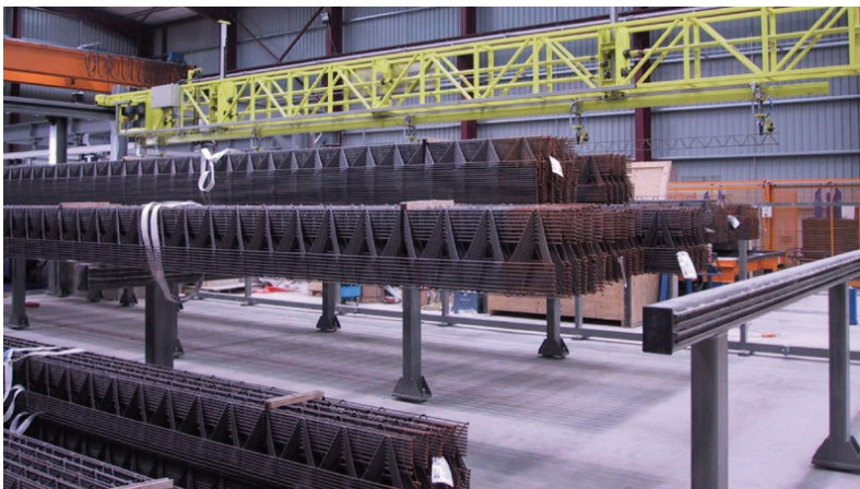
Fig. G.22: Prefabricated reinforcement installed by handling robot (Vollert GmbH + Co. KG, 2006)
