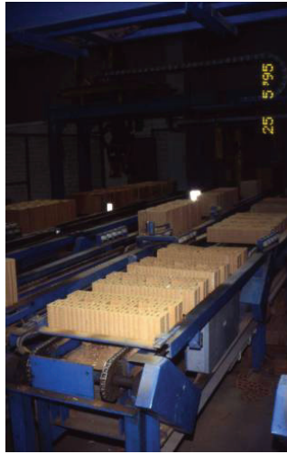
Fig. B.10: decollating station
