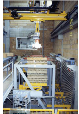
Fig. B.25: de-palletizing system
