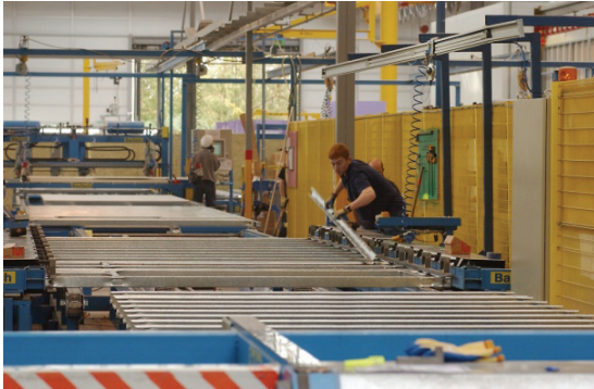
Fig. E.7: Assembly of light steel panels in production
