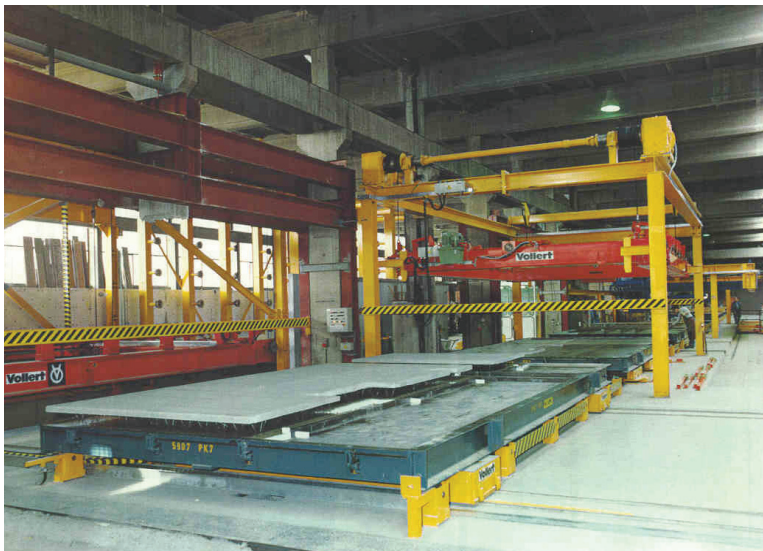
Fig. G.15: Manufacturing ceiling elements using the circuit production method (Vollert Anlagenbau, 1992)
