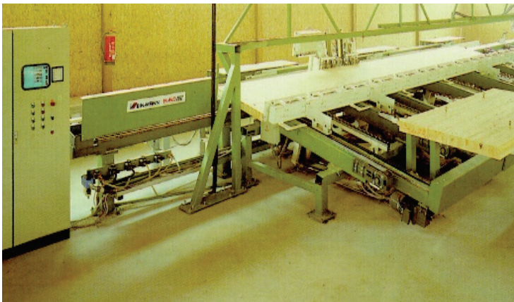
Fig. H.11: Nailing Unit
