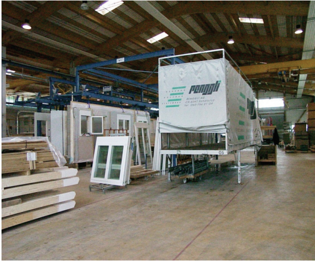
Fig. H.10: Magazine for wall and gabel elements
