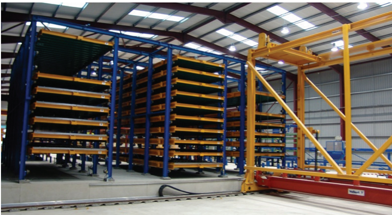
Fig. G.25: Automated horizontal and vertical transport processes (Vollert GmbH + Co. KG, 2006)
