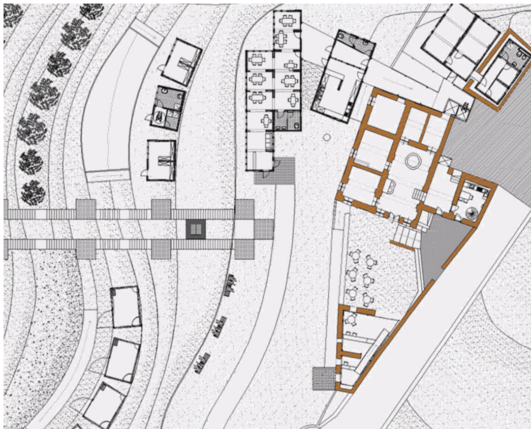
Fig. C.7: The case study of renovation project in Liguria: The new construction is located inside the old stone wall perimeter and along the terracing (GIURDANELA, MARTINA, MORENO, 2004)
