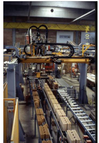
Fig. B.27: robotic assembly system for vertical brickwork layering
