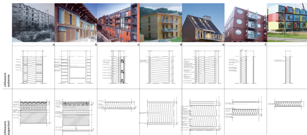
Fig. C.12: Reversible design for housing: The investigation point out methods of construction as a key factor to allow buildings deconstruction and components and materials reclaiming with a selection of residential buildings case studies built with different methods and materials (GIURDANELA, 2008)
