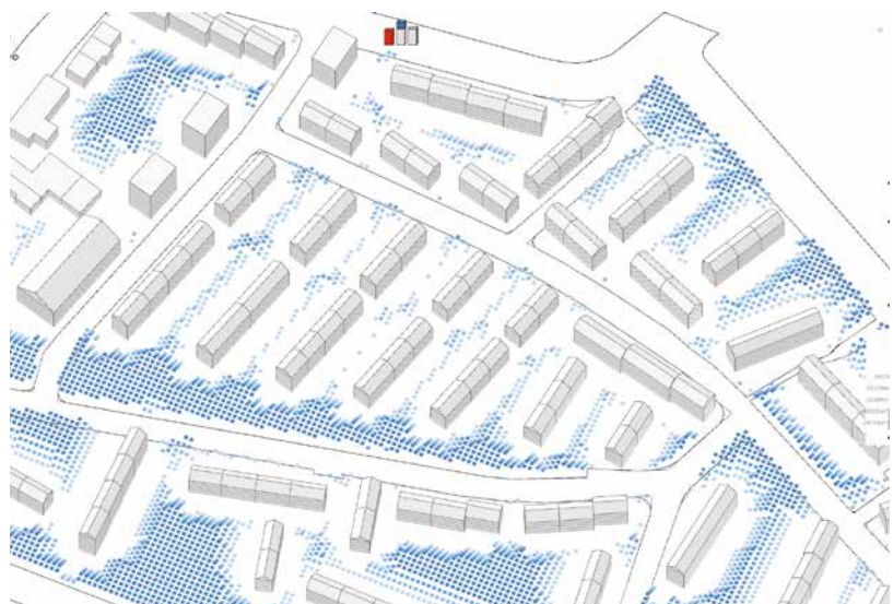
Fig. 1: Creation of an abstract space, showing the maximum possible area to be built on under the assumption of certain building code settings.
