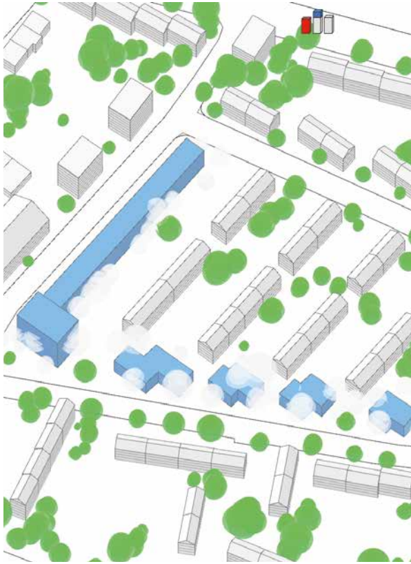
Fig. 2: Design variant with analysis of the existing tree population. (Both figures show fictional buildings and no real design variants created within the project.)
