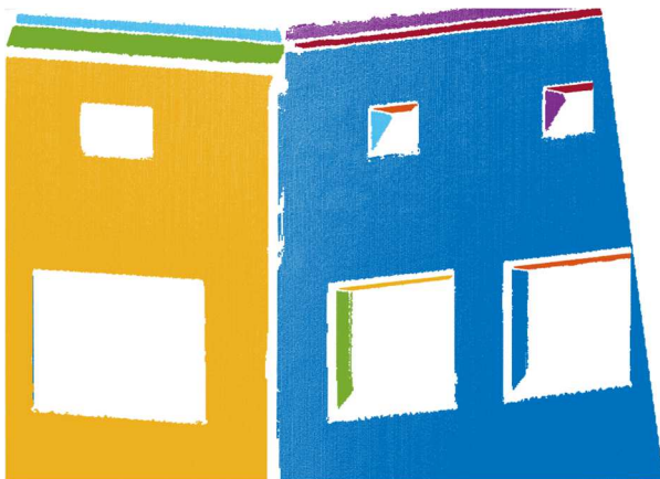
Figure 1. Segmented point cloud of a building facade using a voxel growing algorithm based on local normal vectors.
