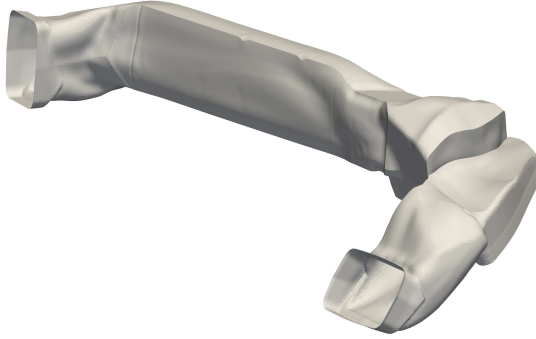
Figure 7.6: Constrained shape optimization of HVAC air ducts with a small filter radius ( r ).
