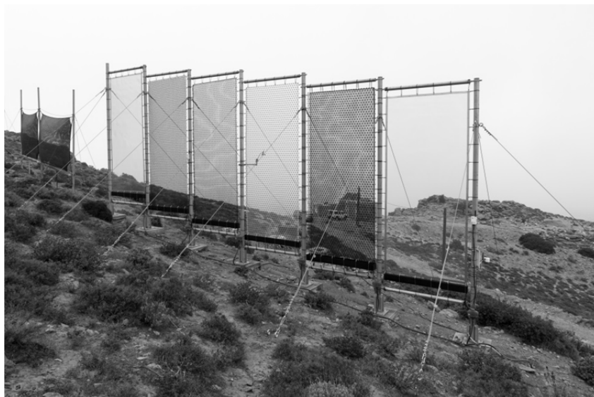
Fig. 1. Photograph of the pilot facility representing the novel fog collector design. Positions 1 through 6 are in sequence from left to right. Positions 1 & 6 are named outside, 2 & 5 middle and 3 & 4 inside. A previously used version of the large fog collector (LFC) can be seen at the left edge of the image.
