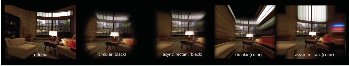
Figure 5.1: Overview of different field-of-view limitation policies compared to the original one as a reference. Both the circular and asynchronous restriction strategies are presented as a snapshot for a fast motion with a high \mathcal{R}_{\max} for the sake of clarity. The remaining parts of the visual field are either filled with black pixels or artificially extrapolated color values, which are less discernible during fast motions. A fading layer is superimposed to smooth the restriction boundaries.
