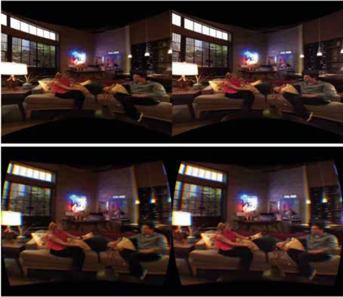
Figure 3.2: Snapshot of a rendered video frame in normal mode (top) and the HMD mode (bottom), where the footage is pre-distorted (HMD lens) such that it can be visualized onto an HMD distortion-free. The omnistereoscopic video sequence is kindly provided by the Fraunhofer HHI [122].
