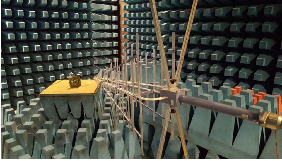
Figure 5.4 The device under test on a rotating table in an anechoic chamber, together with the receiving antenna (from [152]).
