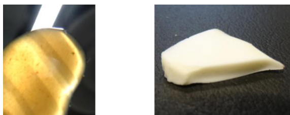
Figure 34: The novel terpene-based biopolymer (left) in comparison to polybutylene terephthalate (right). The amber-colored biopolymer showed a high transparency compared to the white PBT.
