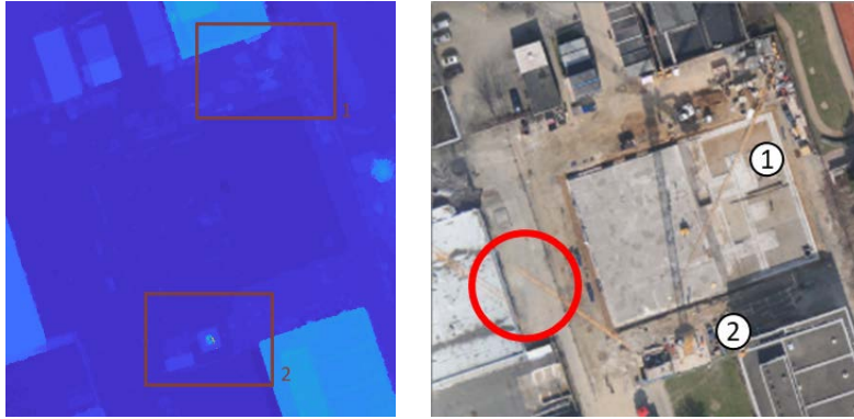
Figure 11: Difficulties with orthorectification of cranes: DSM (left); orthophoto sections with cranes (right)
