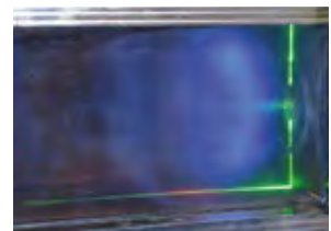
■ Lean-premixed flame with water-injection, visualized by Mie-Scattering
