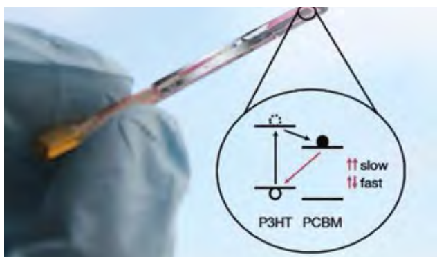
■ Figure: An organic solar cell used for the pEDMR experiments. The inset shows a schematic depiction of the generation of positive and negative polarons via a charge transfer process. The rate of recombination of the two polarons depends on the fraction of polarons with anti-parallel spin orientation and thus can be manipulated by magnetic resonance.
