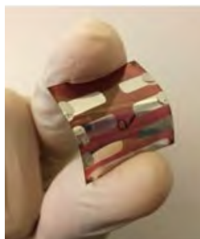
■ Fig. 2: ITO-free flexible organic solar cell
