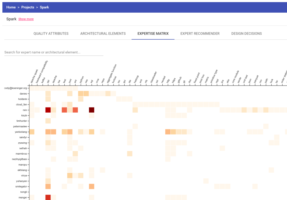
Figure 5.40: Expertise matrix viewpoint: rows correspond to individuals, columns capture architectural elements, and cells indicate the expertise of an individual on the corresponding architectural element
