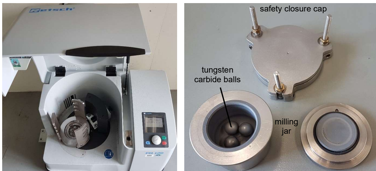
Figure 2.1. Ball-mill (left) and milling jar (right) with safety closure cap and tungsten carbide balls.
