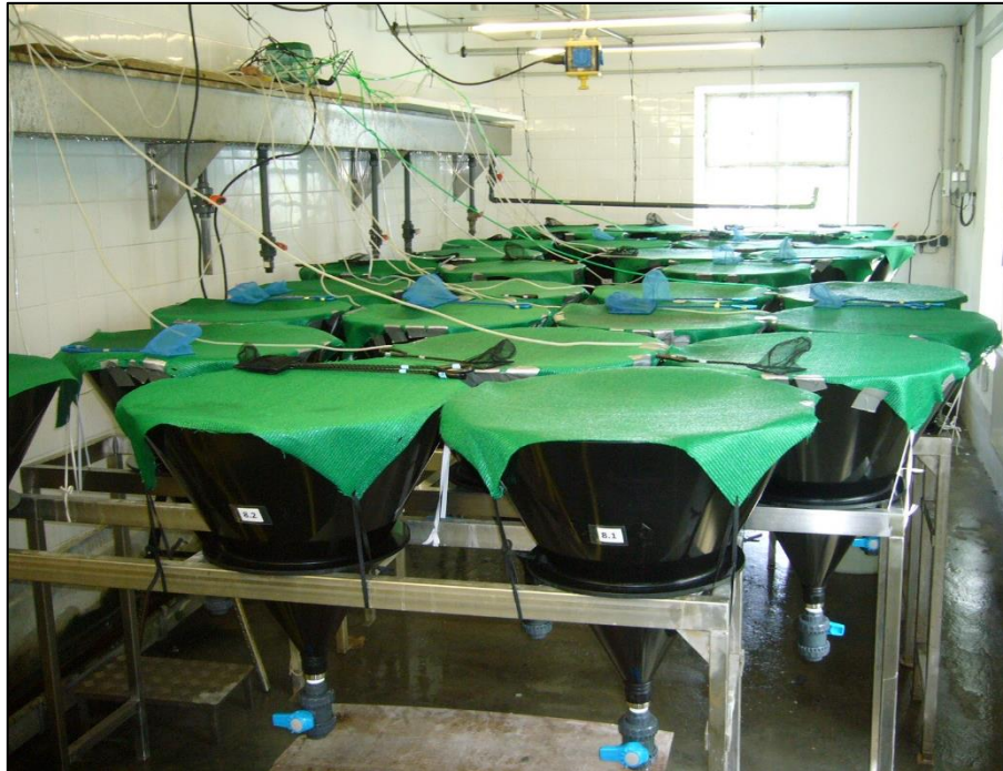
Figure 2.1: Experimental setup post-infestation. Funnel-shaped holding units with covering containing fish (infested and control individuals) after the infestation process. Holding units were randomly placed in special racks for a better handling, aerated by pump or provided by a constant flow of water.
