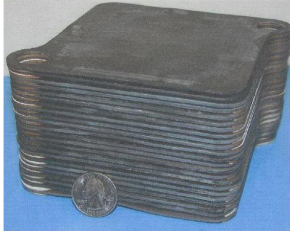
Figure 2.11: Ceramic microchannel recuperator matrix from Cermatec Inc [113]
