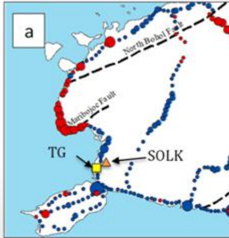
(a) Land uplift (red) and land subsidence (blue) from geodetic levelling (Flores, Madjus and Reyes, 2017)
