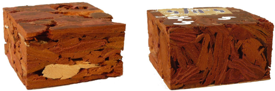
Fig. 3 Bark panel with horizontal and vertical particle orientation ( 28 \times 50 \times 50 \text{ mm}^3 , density 450 \text{ kg/m}^3 )
