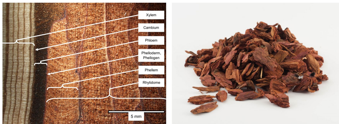
Fig. 1 Cross section of a larch tree bark layer and particulate bark material
