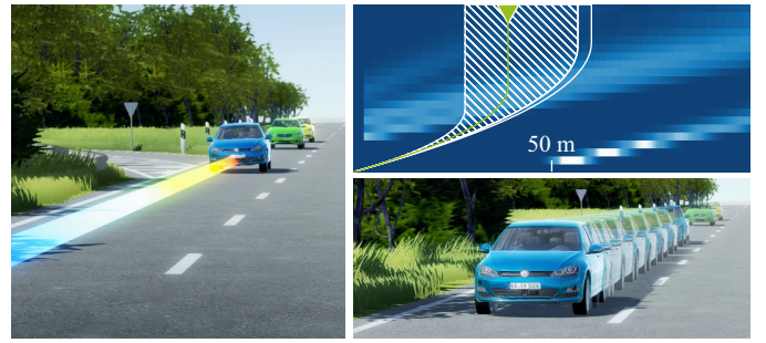
(a) In this continuation of the scenario in Fig. 2, the ego vehicle stayed operational until entering the highway. Once it has reached zero steering angle, it can pick a gentle deceleration to minimize the risk of a rear-end collision. In the simulated failure, the vehicle fails while the valve is in motion (the hatched area). Since the transition to a gentler deceleration here continuously increased safety, it was not masked as described in Sec. II-B3.
