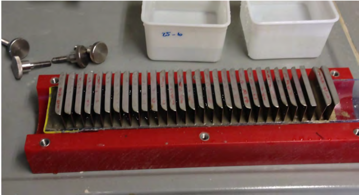
Fig. 1.13: Sediment core division of GOSED06: half of the sediment core was portioned with cutting plates in 1 cm samples.
