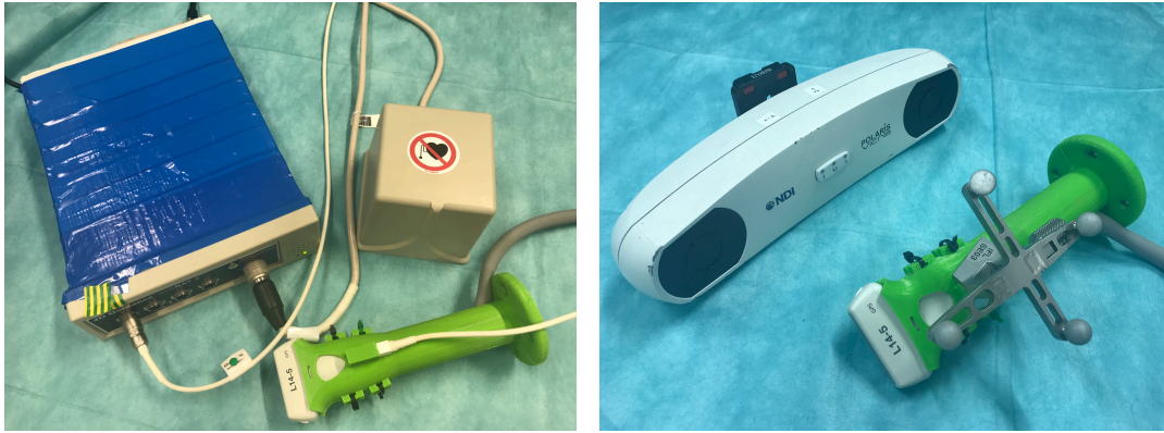
Fig. 2.3. Tracking devices for free-hand 3D ultrasound. Left: an EM sensor is attached to an ultrasound linear transducer (white element inserted in the green casing), an EM field is emitted by the generator (cube on the top right) and the sensor position with respect to it obtained. Right: An optical marker is attached to the transducer, while an external camera emits infrared signals and captures their reflections from the marker's spheres.
