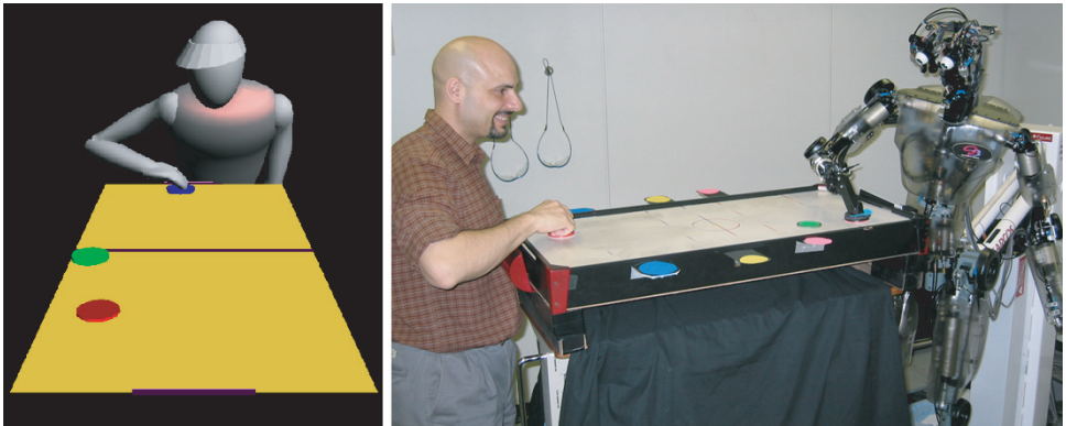
Fig. 2. Simulated air hockey (left) and playing air hockey with a humanoid robot (right). In the simulated game the disc shaped object near the centerline is a puck that slides on the table and bounces off the sides, and the other two disc shaped objects are the paddles. The virtual player controls the far paddle, and a human player controls the near paddle by moving the mouse. The object of the game is to score points by making the puck hit the opposite goal (the marked area at the ends of the board). In the physical game the paddles are held by the human and the humanoid robot, and the puck is about to be hit by the robot.
