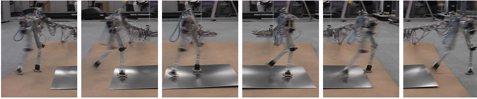
Fig. 11. Snapshots of a walking experiment over surfaces with different friction properties and a seesaw-like metal plate with a slight change in the slope. Also see the plots in Figs. 12–14 for joint trajectories, torque commands and stepping period for this experimental run, respectively.
