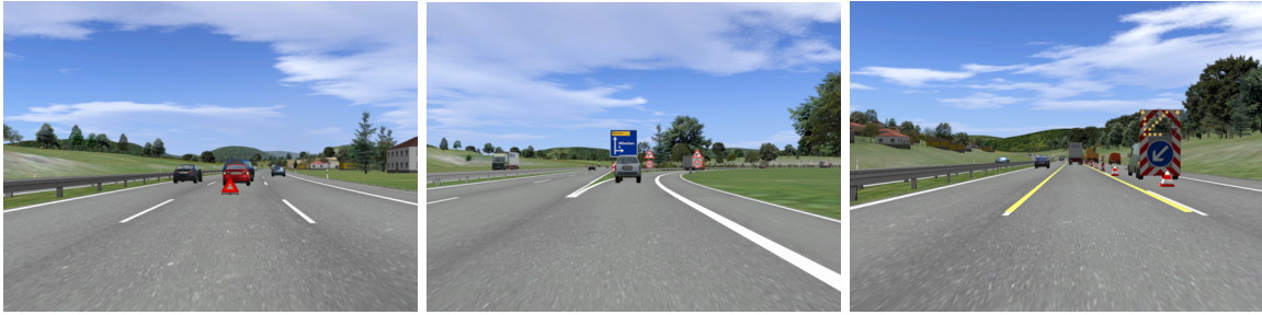
Figure 5.3: The three take-over situations, the construction site, the interstate crossing and the crash site (left to right). The figures show the take-over situation only few meters prior to the system limit.
