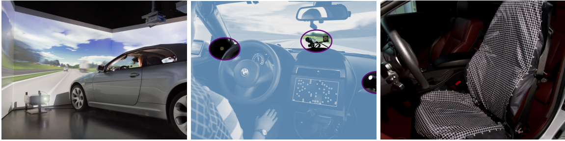
Figure 4.3: The figures show, from left to right, the simulator and the vehicle mockup, the three cameras of the eye-tracker SmartEye and the seat pressure mats and their implementation in the vehicle. Figures with friendly permission by Fabian Marco Fischer.
