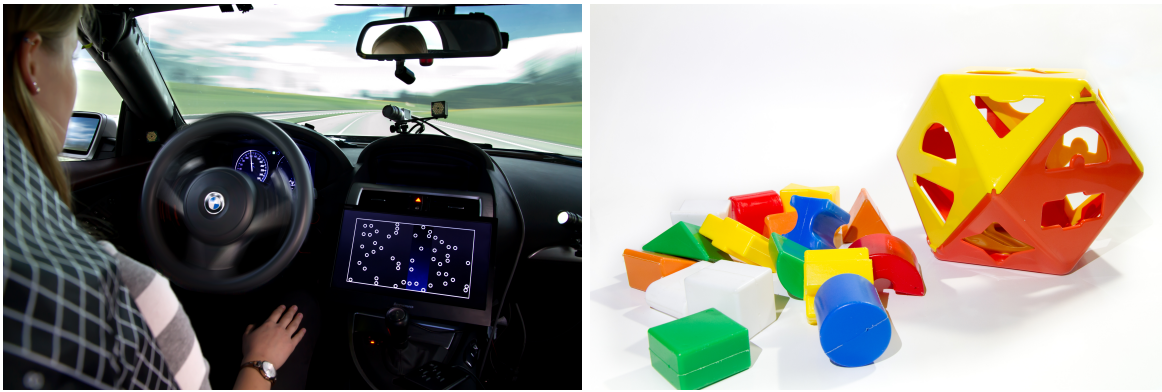
Figure 6.2: The left figure shows the SuRT in the center console of the vehicle. The right figure shows the shape-sorter ball that was put into a fabric bag with openings during the experiment to only allow manual (and not visual) interaction during the task. Figures with friendly permission by Fabian Marco Fischer.
