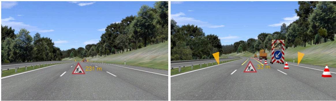
Figure 9.2: The construction site with the additional HMI at the moment of the Rtl (left) and 33 meters away from the system limit (right) viewed through the windshield.
