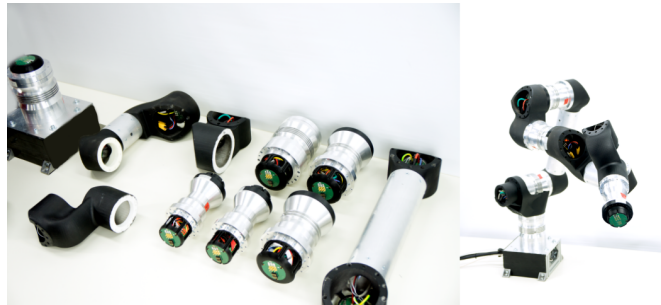
Fig. 1. proModular.1 is a set of modules (left) that can be composed into an industrial robot (right).
